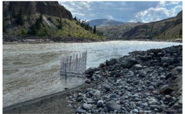
SONAR installed on the Fraser River at Churn Creek Aug 24-25 to monitor salmon migration in the Fraser between Big Bar and the Chilcotin River
